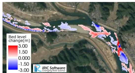
Fig.14 Analyzed result of bed level change after a large-scale flooding ( $Q_{peak}=10,000\text{m}^3/\text{s}$ )
