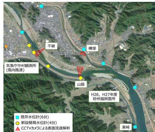
Fig.7 Observation system of water level and CCTV camera during flooding
