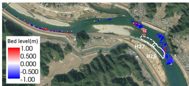
Fig.10 Measured riverbed level change before and after the flood of Sept. 2015
