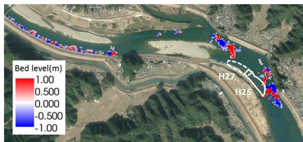
Fig.11 Analyzed result of riverbed level change before and after the flood of Sept. 2015
