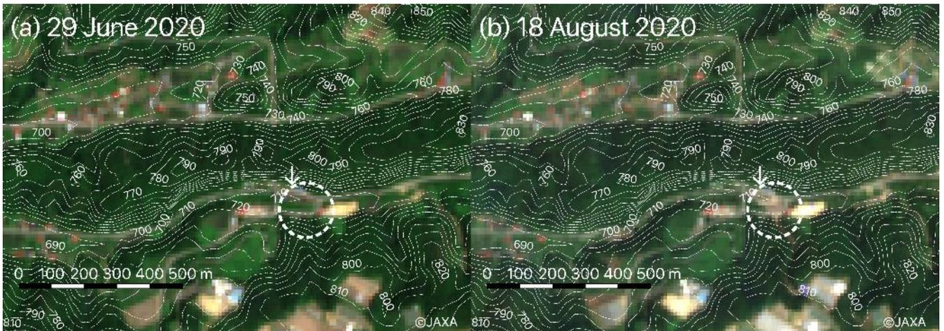
**Fig.5** RGB composite images of Taki-machi observed on (a) 29 June 2020 (before torrential rains) and (b) 18 August 2020 (after torrential rains). Arrows show the approximate location of the photograph in Fig.4(b). Images were obtained from Sentinel-2A/B satellites, and we used the Sentinel Application Platform (SNAP)<sup>48)</sup> for atmospheric correction. We used the AW3D30 digital surface model with a 30 m spatial resolution<sup>32)</sup>. White contour lines are at 10-m intervals.
